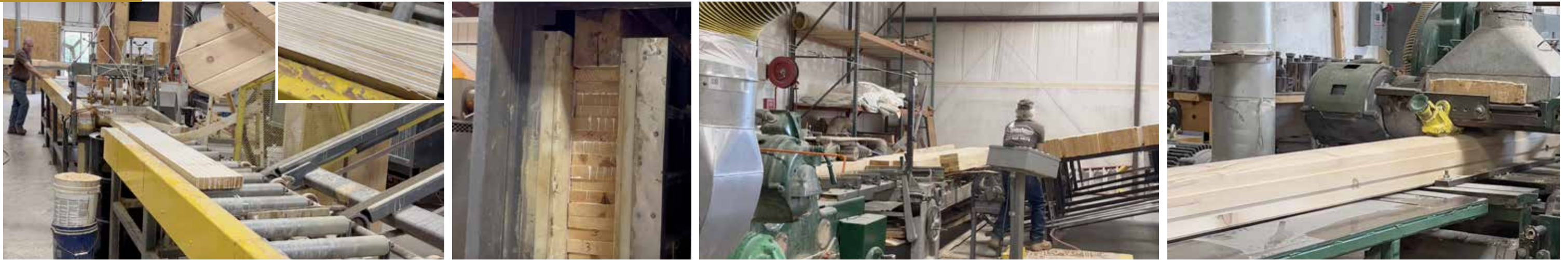
LEFT TO RIGHT Adhesive is applied to the milled ply. The boards are stacked and compressed, then bonded and cured. The engineered cants are fed into the planer where they are prepared for cutting. Using four cutting heads, each log is shaped per the plan's specs.
